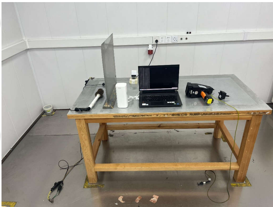
Electrostatic discharge Test Setup-1
