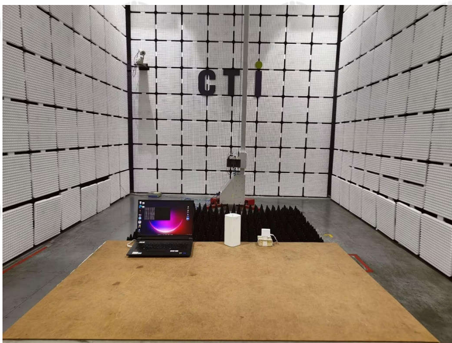
Radiated emissions Test Setup-1
