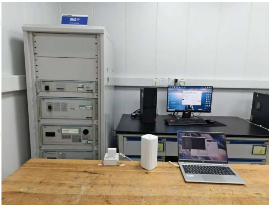
Voltage dips and interruptions Test Setup-1
