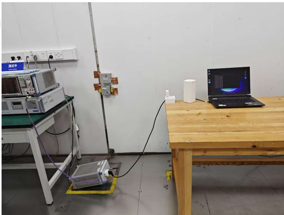
Conducted emissions Test Setup-3
