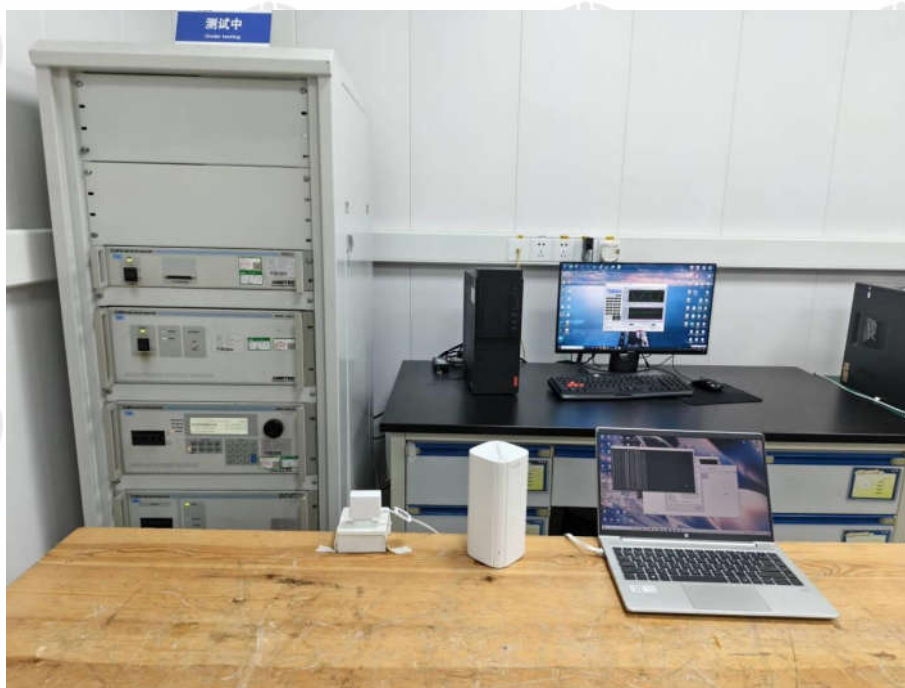
Voltage changes voltage fluctuations and flicker Test Setup-1
