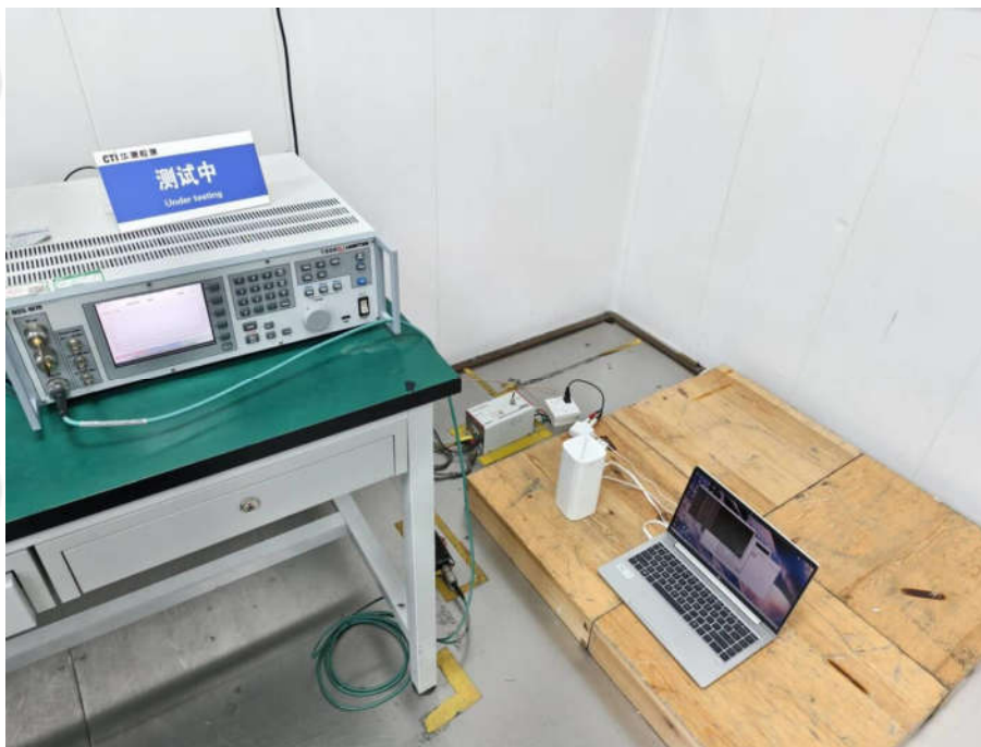
Continuous induced RF disturbances Test Setup-1
