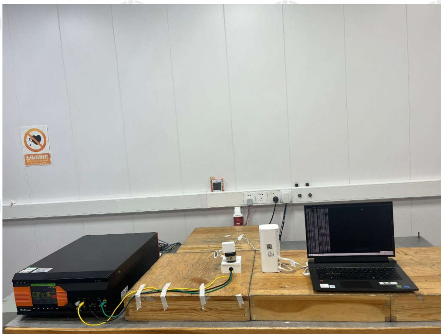
Electrical fast transients burst Test Setup-2
